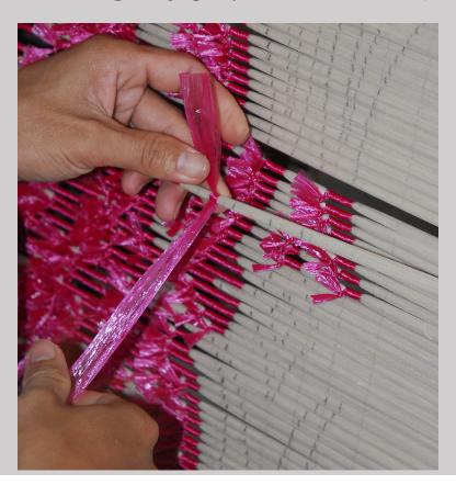
Figure 6.5c Tying thread bundles at Pertenunan Berdikari Handwoven Cloth Factory in Singaraja, Bali, Indonesia (photograph by Carol Ventura, 2007).
