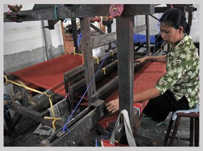
Figure 6.5e **Weft ikat** woven on a **foot loom** at the Pertenunan Berdikari Handwoven Cloth Factory in Singaraja, Bali, Indonesia (photograph by Carol Ventura, 2007).
