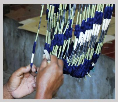
Figure 6.5d Removing the binding from dyed thread bundles at Pelangi in Sideman, Bali, Indonesia; (photograph by Carol Ventura, 2007).
