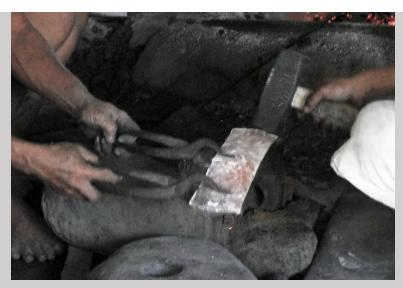
Figure 6.9e Forging a red-hot brass gangsa key at Gong Yudha, Tihingan, Bali, Indonesia (photograph by Carol Ventura, 2007).
