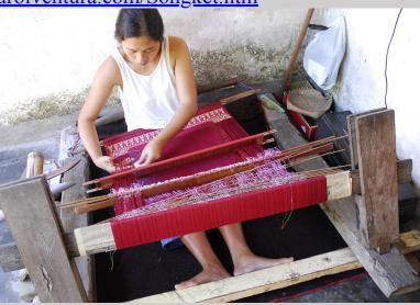
Figure 6.4b Supplementary metallic weft is inserted in Sideman, Bali, Indonesia (photograph by Carol Ventura, 2007).
