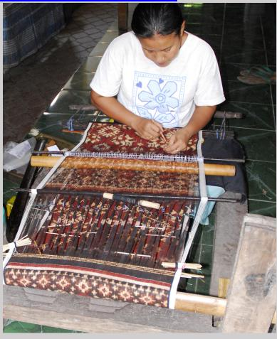
Figure 6.5f Using a pick to adjust the warp and weft while weaving double **ikat** geringsing on a body-tensioned loom in Tenganan, Bali (photograph by Carol Ventura, 2007).
