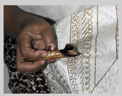
Figure 6.2c Applying hot wax with canting tool over pencil lines at Galeri Batik Kuno Danar Hadi, Surakarta, Java, Indonesia (photograph by Carol Ventura, 2007).
