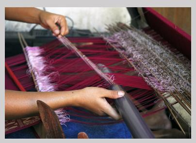
Figure 6.4d The shed is changed again by releasing the tension by moving slightly forward while pulling up the next string heddle rod (photographs by Carol Ventura, 2007).
