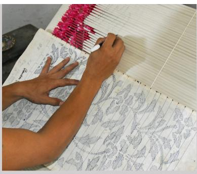
Figure 6.5b Following a graphed pattern to precisely mark weft bundles at Pertenunan Berdikari Handwoven Cloth Factory in Singaraja, Bali, Indonesia (photograph by Carol Ventura, 2007).
